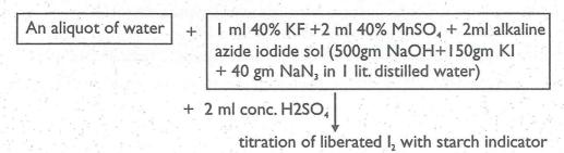
DO ( mg/L ) = (A X N X 8000)/ B A= ml of Na<sub>2</sub>S<sub>2</sub>O<sub>3</sub> B= ml of water sample taken N= Normality of Na<sub>2</sub>S<sub>2</sub>O<sub>3</sub>
